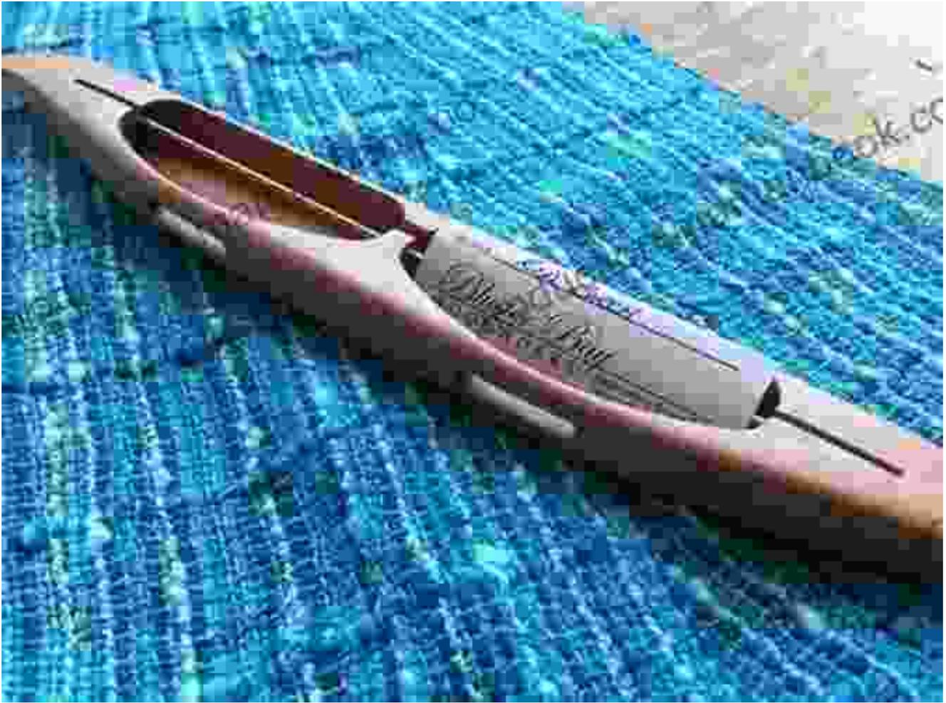
The shuttle is a tool used to insert the weft thread between the warp threads. Swedish weaving often employs two shuttles, one for each color or type of weft yarn used in the pattern.
